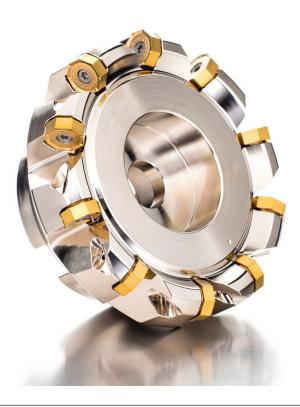
A new highly economical and productive face mill utilising two types of double-sided negative inserts. Economical octagonal ON..06 inserts with 16 cutting edges and APMX of 4 mm, and productive square SN.. 17 inserts with 8 cutting edges and APMX of 7 mm. Shell style (DC = 50 - 250 mm) available with differential tooth pitch. Body treated for longer tool life.
